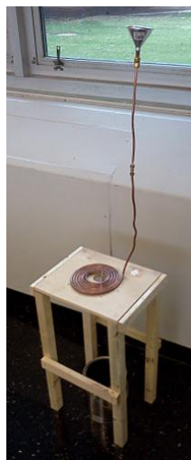
Figure VII.iii.3 Heat dissipation coil experiment setup.
